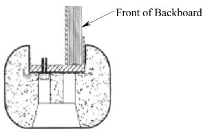
Figure 1: Holes Drilled Through Frame - Towards Rear of Board
