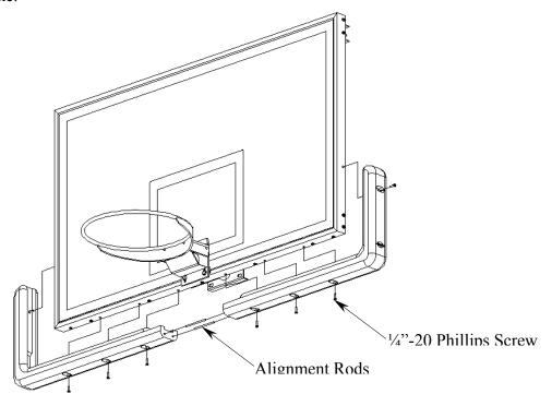
Figure 2: Assembly of Edge Pad Onto Backboard
