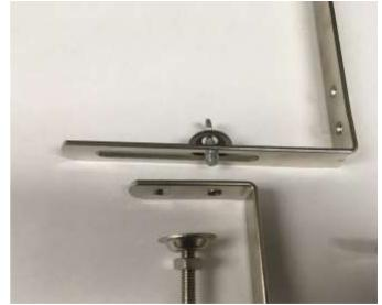
Tighten the thumb screw to secure the "L" bracket to the clamp to create a net support.
