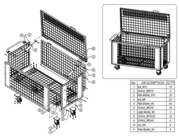
1. Attach the bottom panel to the side panels (These are the long panels)
