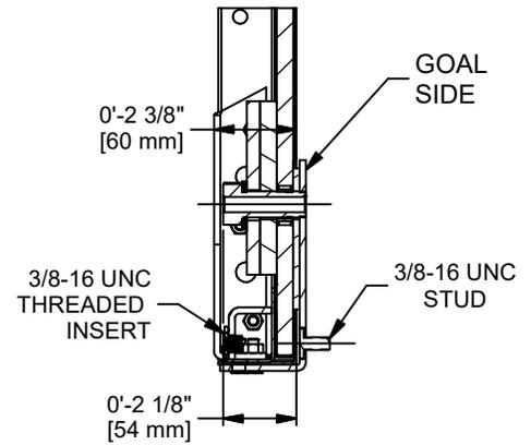
MATERIAL IS 1/2" THICK TEMPERED GLASS WITH STEEL FRAME
