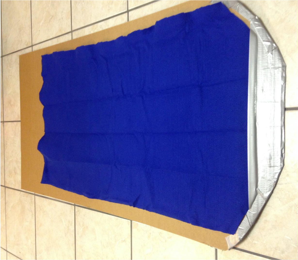
Flipped to bottom, cut felt slightly less than width, secured front end of felt to angled portion of lip.
